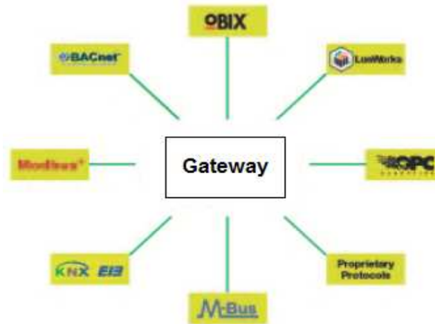
Fig. 2 – Gateway using several protocols
